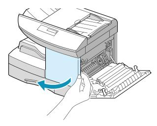
**3** Pull down the fuser lever. This will release pressure on the paper.
